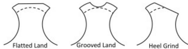
The application of relief types and amounts are dependent on many factors such as material properties being tapped, style and size of tap, how the tap is being used (hand, machine, etc.) and application requirements. By providing us with as much information about your tapping application as you can, it will enable our engineers to design a tap with the proper relief.
